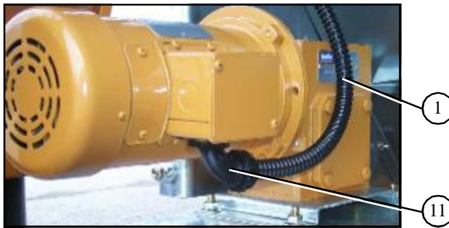
Meter roll speed sensor and rear discharge switch conduit. This is a photo of the front section of the conduit that runs through the gussets on the left side of the dryer.
